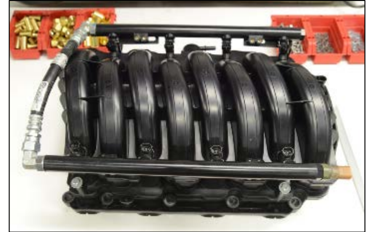
5.3L manifold & PFI Fuel Rails
